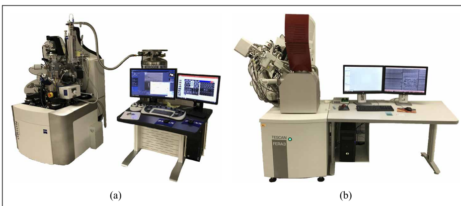
Figure 2. (a) Scanning electron microscope. (b) Focused ion beam. Note that attacker does not need to purchase all these instruments since rent by time is quite low cost.
