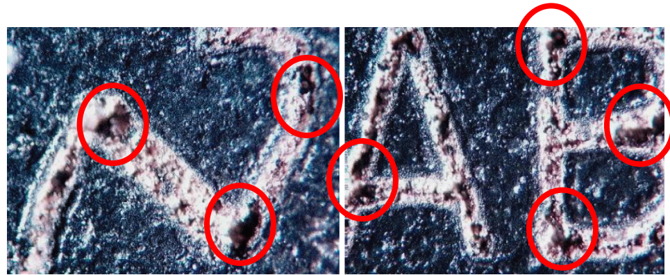
Burned markings from low quality laser
