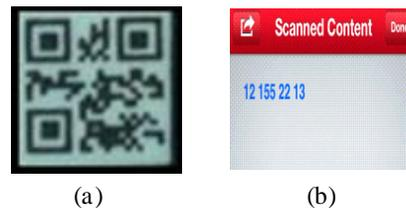
Fig. 2 (a) enlarged QR code taken using the iPhone 4 camera; (b) scanned QR Code depicting the encrypted and compressed data using the iPhone SCAN Application.
